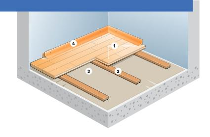
The Unobat 45 System is a low profile, high performance batten based system. It is designed for use over flat subfloors.
