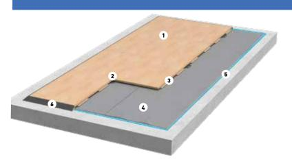
The Arena Master Portable Sports Floor comprises of 22 mm solid hardwood floorboards, prefabricated into lightweight panels.
