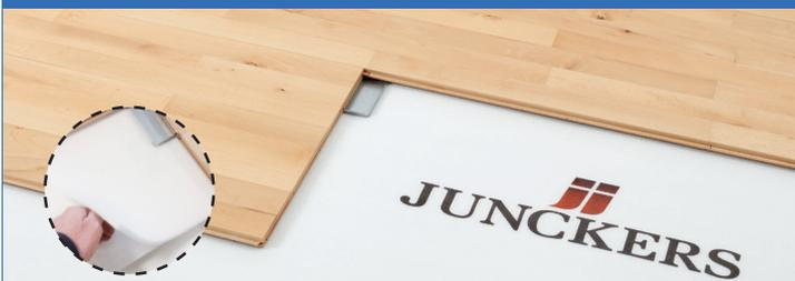
The panels are installed floating on a 10 mm Sports foam. The intermediate layer of foam is required to provide correct shock absorption and resilience.
